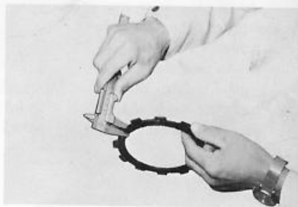
Fig. 6-12-3 Measuring drive plate thickness
