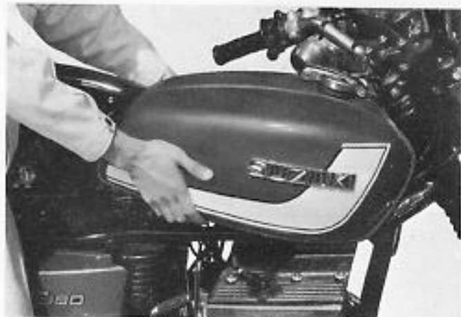
Fig. 6-1-2 Removing fuel tank
