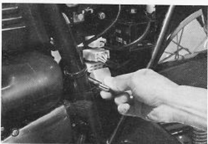
Fig. 6-1-4 Disconnecting alternator wires
