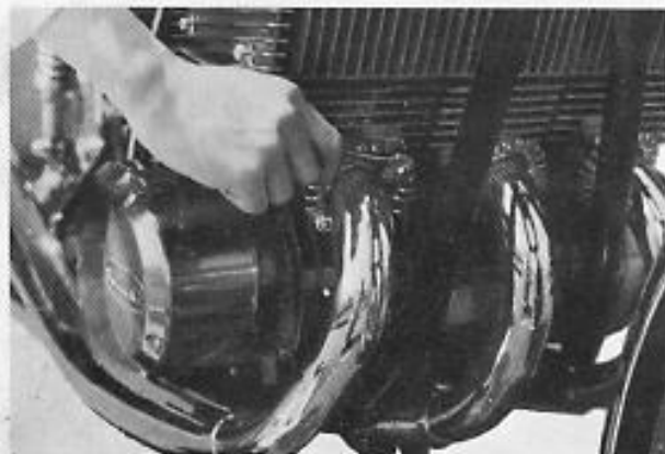
Fig. 6-1-17 Removing exhaust pipe clamp
