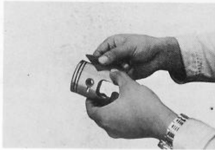
Fig. 6-6-4 Polishing piston surface
