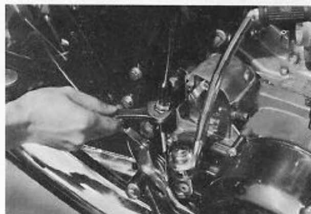
Fig. 6-1-14 Removing rear brake lamp switch
