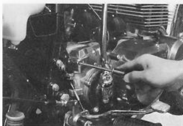
Fig. 6-1-10 Removing oil pump cover
