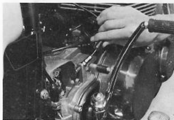
Fig. 6-1-12 Disconnecting oil pump control cable
