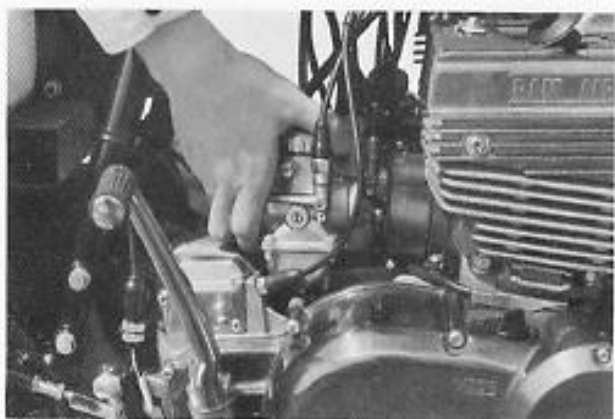
Fig. 6-1-9 Removing center & right carburetor
