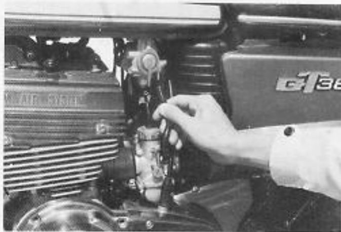
Fig. 6-1-1 Disconnecting fuel pipe
