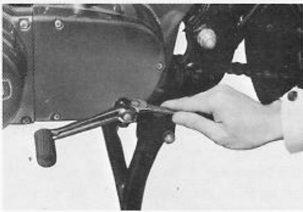
Fig. 6-1-23 Removing gear shift lever
