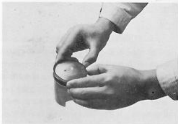
Fig. 6-5-1 Removing piston ring
