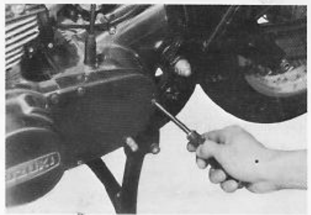
Fig. 6-1-24 Removing engine sprocket outer cover
