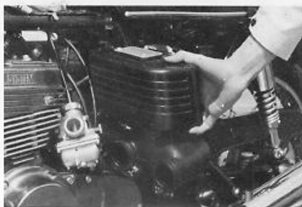
Fig. 6-1-8 Removing air cleaner
