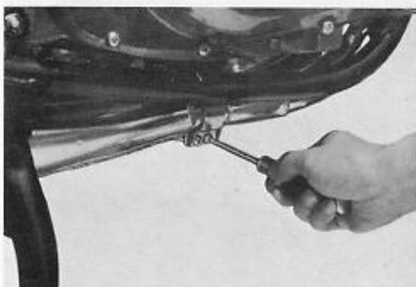
Fig. 6-1-20 Loosening muffler connector clamp
