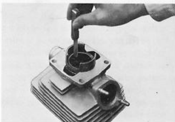
Fig. 6-5-3 Measuring end gap
