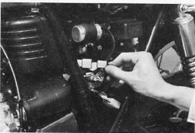
Fig. 6-1-5 Disconnecting breaker wires
