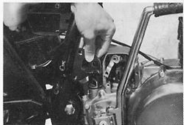
Fig. 6-1-28 Removing engine mounting plate
