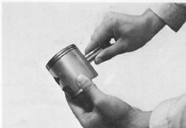
Fig. 6-6-3 Inspecting piston pin holes
